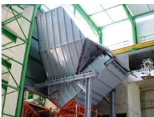
Ram feeder For pushing the product onto the cutting tools
