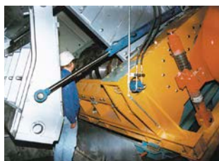
Ejection door For easy removal of unshreddable parts
